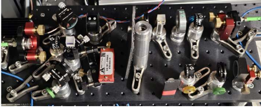
Figure 6.6: Photograph of the double-pass AOM setup which switches on the CW reference beam during the stabilization period.
